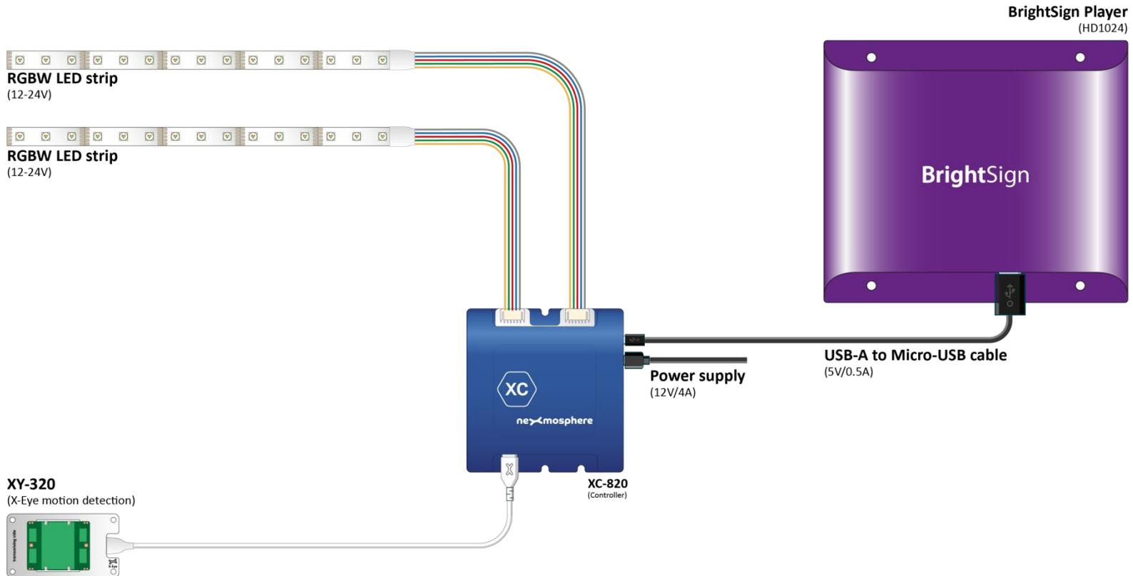
Sensors ① | ④ Motion sensor and 2 RGBW LED strips
